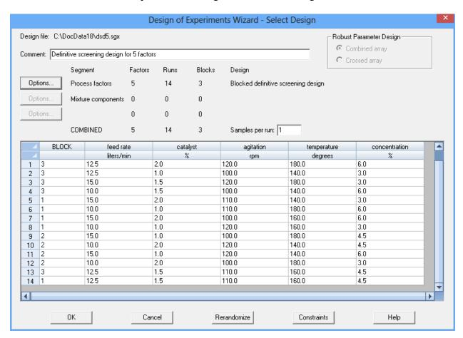
There are a total of n = 14 runs with each factor at 3 levels. The blocking pattern has been selected following the methods of Jones and Nachtsheim (2012) which uses the D criterion to pick an optimal design.
