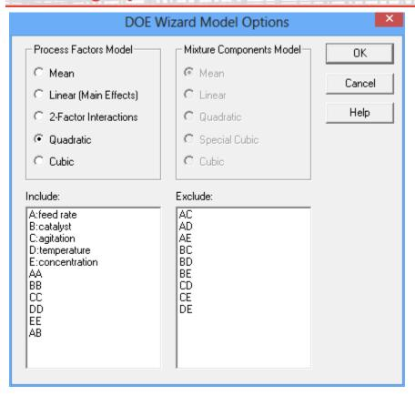
It contains 5 main effects, 5 quadratic terms, and 1 two-factor interaction. The selected interaction is completely arbitrary and is partially confounded with all of the other two-factor interactions.
