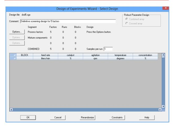
Since all of the factors are controllable process factors, only one *Options* button is enabled. Pressing that button displays a second dialog box:
