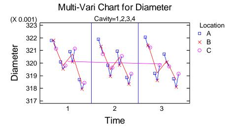
Each plotted point is now the average of the two *Samples* plotted previously. If more factors are removed, the data is averaged over all levels of the removed factors.
