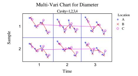
A row of plots is displayed for each *Sample*, with *Time* increasing along the horizontal axis. Each section of the plot shows the measured *Diameter* at three locations on *Parts* from each of the four *Cavities*. Lines connect:
